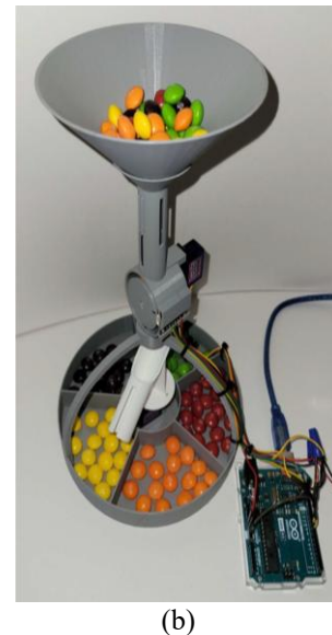
Fig. 1. (a) Functional Modules of the Automated Sorting Device; (b) Photograph of the Prototype Sorting Device.
